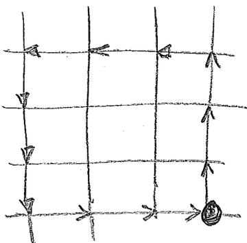
The same sequence of steps around dislocation will lead to displacement  $\vec{b}$
