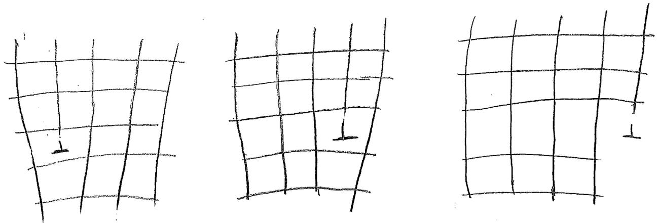
If dislocation moves through the crystal it produces shift of the upper half crystal by the unit vector  $\vec{b}$ . The shear that leads to the dislocation motion is much smaller than  $\mu$ . That is why  $\gamma_m \ll \mu$
