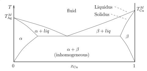
*Note*: Most alloys have a melting range, where a solid phase coexists with a liquid of both components. The limits of this range are called solidus and liquidus.
