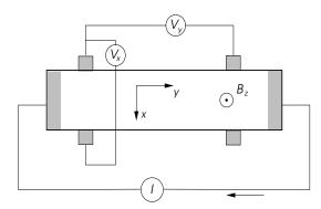
Figure 4.3: Schematic view of a Hall bar. The current runs a long the y-direction and the magnetic field is applied along z-direction. The voltage  $V_y$  determines the conductance along the Hall bar, while  $V_x$  corresponds to the transverse Hall voltage.
