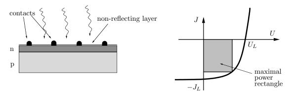
Figure 2.13: Solar cell design and shifted current-voltage characteristics. The efficiency is maximal for a maximal area of the power rectangle.
