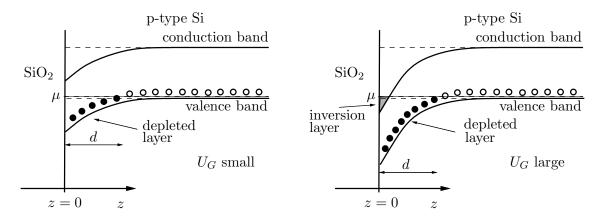
Figure 2.15: Depletion layer at the  ${\rm SiO_2}$ -Si interface for  $0 < e\,U_G < E_g$  (left panel) and the inversion layer  $E_g < e\,U_G$  (right panel).
