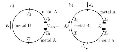
Figure 6.8: Schematics of thermoelectric effects. On the left panel (a) a representation of Seebeck effect is given, where the symbol E is used instead of  $\mathcal{E}$ . On the right panel (b) the Peltier effect is represented. In our analysis, both systems were effectively one-dimensional.
