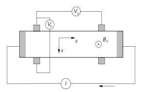
Figure 4.4: Schematic view of a Hall bar. The current runs a long the y-direction and the magnetic field is applied along z-direction. The voltage  $V_y$  determines the conductance along the Hall bar, while  $V_x$  corresponds to the transverse Hall voltage.
