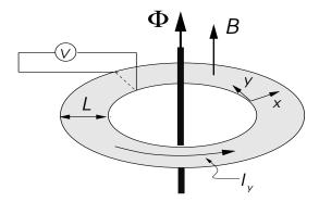
Figure 4.8: Corbino disk for Laughlin's argument. According to the Hall bar in Fig. 4.4, the radial (transverse) component of the Corbino disc is denoted by x, while the angular (longitudinal) component is termed as y. Both the homogeneous magnetic field B and the flux  $\Phi$  point along the z-axis perpendicular to the plane of the disc.
