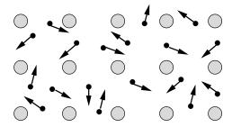
Figure 1: Atom cores and the surrounding electrons.
