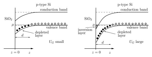
Figure 2.15: Depletion layer at the SiO<sub>2</sub>-Si interface for  $0 < e\,U_G < E_g$  (left panel) and the inversion layer  $E_g < e\,U_G$  (right panel).
