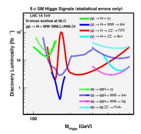
Plot based on "optimistic" (and realistic!) simulations from ATLAS and CMS for the LHC with 14 TeV (at 7 TeV one needs about a factor  $\sqrt{2}$  more luminosity)
