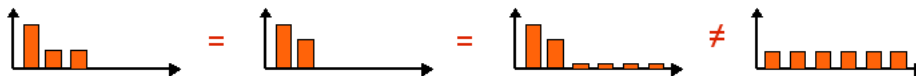
Figure 2: The min-entropy only cares about the peak probability, that expresses the probability of taking a correct guess in a single shot approach, ignoring how the other the probabilities are spread.
