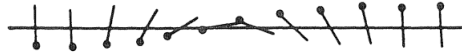
Figure 3.3: Pegs on a line representing the kink (soliton) solution to the sine-Gordon equation.
