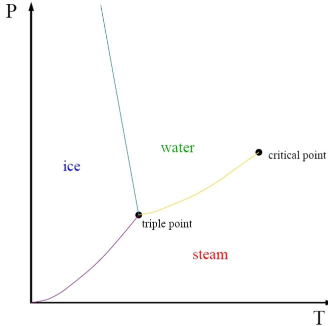
Figure 1: The phase diagram of water. (Taken from [3])
