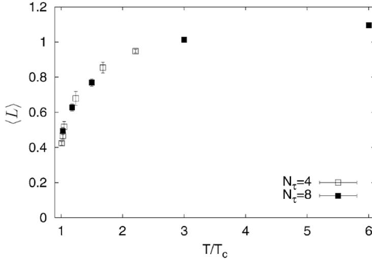
Figure 6: The expectation value of the Polyakov loop as a function of the temperature. The spatial lattice size is  $N_s = 32^3$ . The expectation value is zero below the critical temperature  $T_c$ . The graph and the data are taken from [5]
