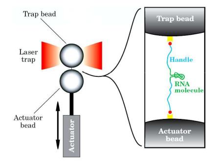
Difference in positions of the bottom and top beads as control parameter.
